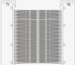
40 beam parallel pattern generated by Model 841
